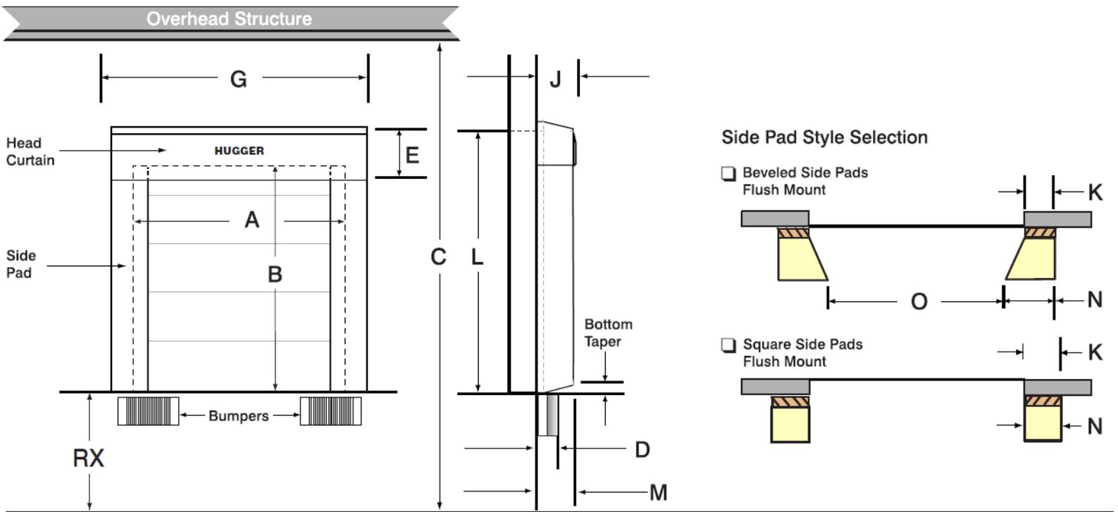
Note: If the seal is incorrectly specified and/or misapplied for the application, not only will the seal be ineffective, but it may result in damage to the building and the dock seal. Apply taper to dock seal according to the slope of approach to the dock, i.e. dock seal taper should be considered for each 1% angle of decline/incline, over 2%.
